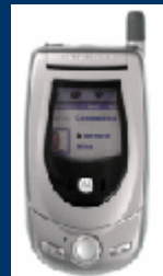
Motorola A760 Linux/Java handset/PDA Mobile phone, PDA, digital camera, video player, MP3 player, speakerphone, messaging, Internet access
